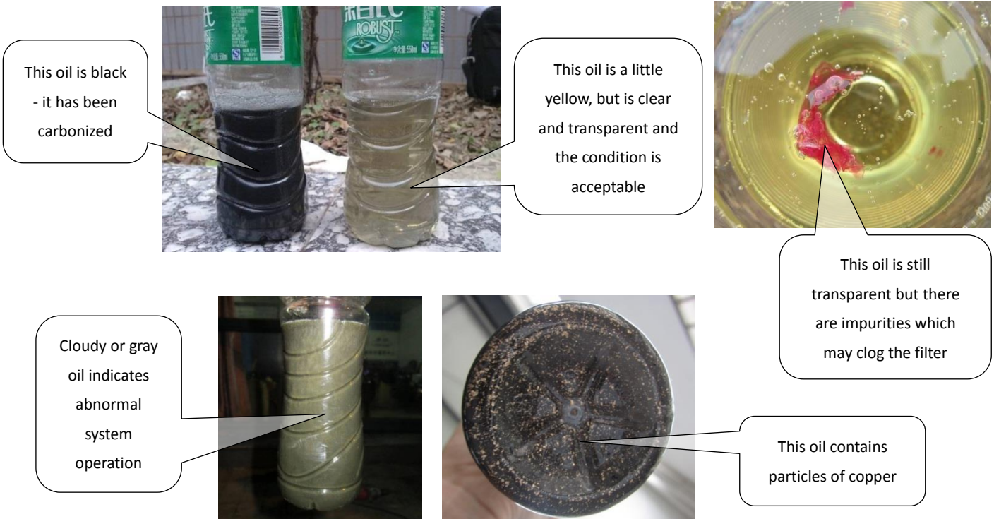
Figure 3: Inspecting compressor oil
