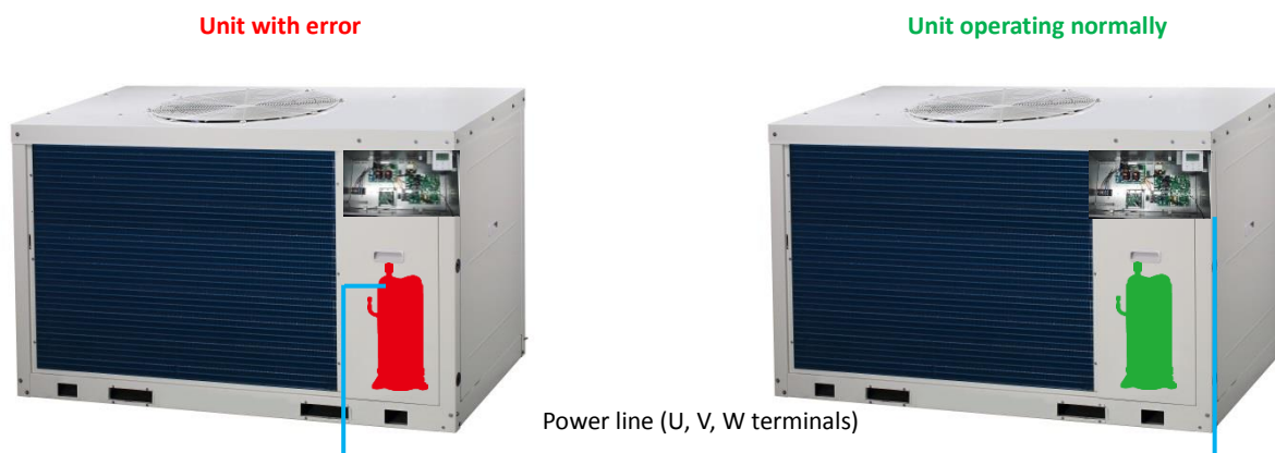
Figure 1: Connecting compressor to an error-free unit
