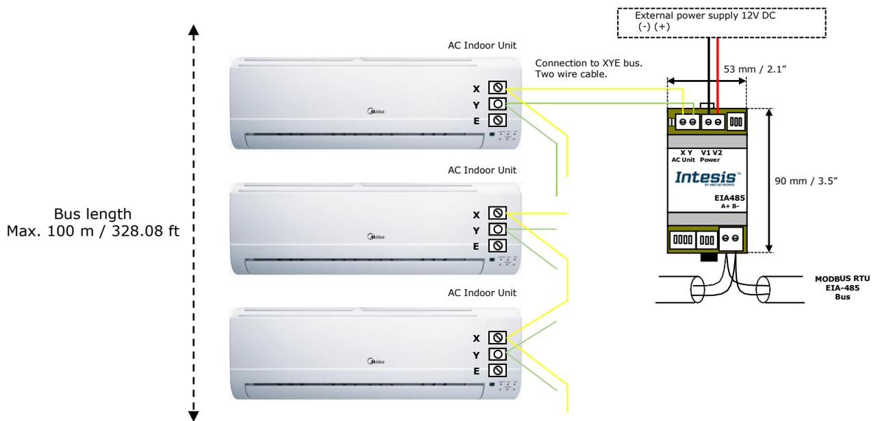
Figure 2.2 INMBSMID004I000 / INMBSMID008I000 / INMBSMID032I000 connection diagram
