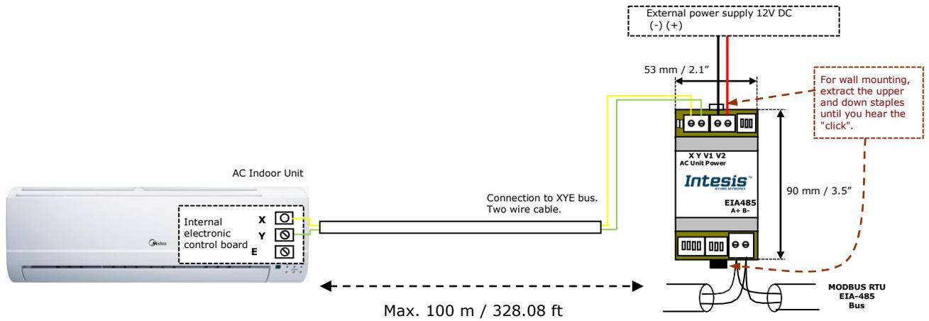
Figure 2.1 INMBSMID001I000 connection diagram
