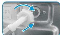
Connect the water supply hose to the water inlet valve and a water tap with cold water as indicated.
