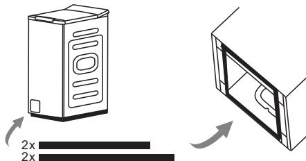
1. Get the machine laid on the floor, using some soft material like foam or clothes between the machine and floor for a protection;
